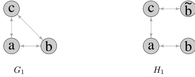
Figure 4: Node b is split by adding node \tilde{b} \notin \mathcal{V}_G and replacing edges \{(b, c), (c, b)\} with \{(\tilde{b}, c), (c, \tilde{b})\} .
